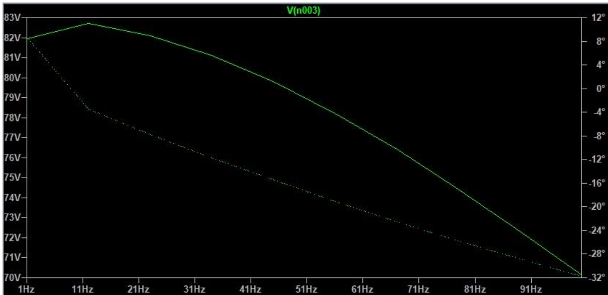
[Figure 4.1.20: AC frequency sweep of low-end adjustable gain non-inverting amplifier, R12 (R4 in simulation) set to 1k\Omega ]
