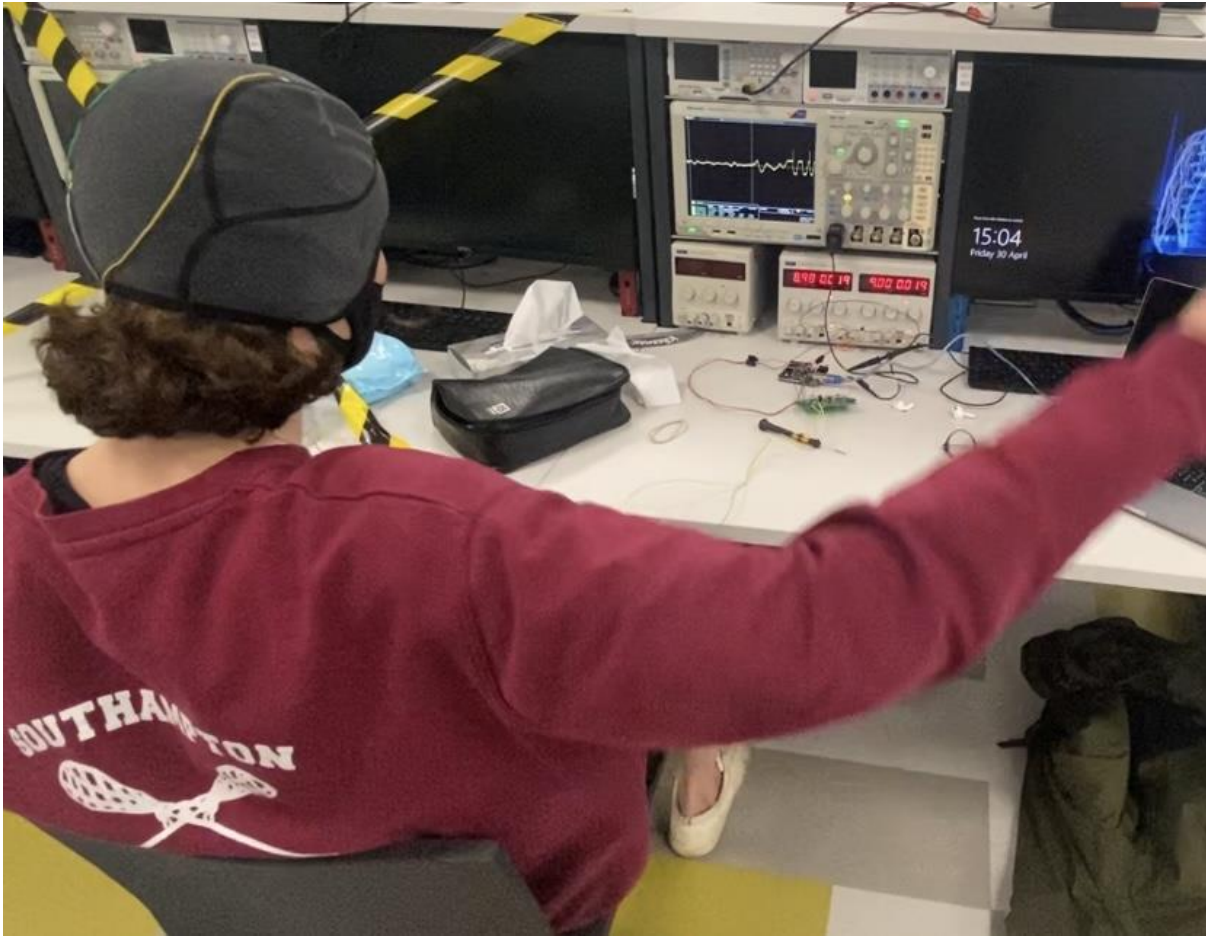
[Figure 4.3.2: System test with arm at 90 degrees to body and active showing voltage spikes due to motion]
