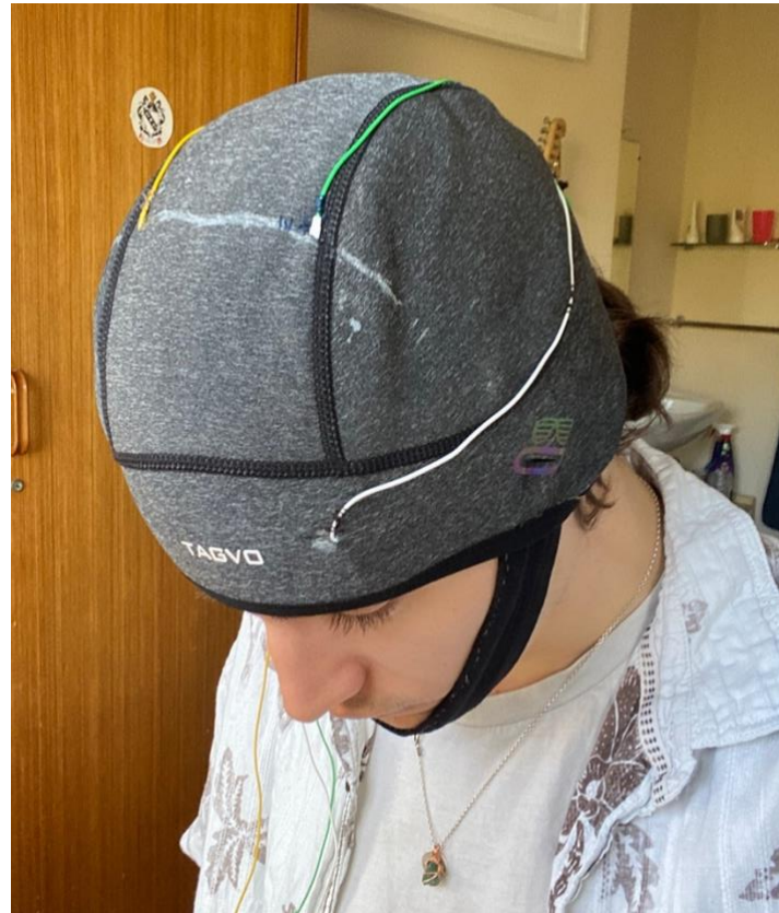
[Figure 4.2.3: Electrodes situated on the scalp in positions corresponding to the cortical motor regions of the arms]
