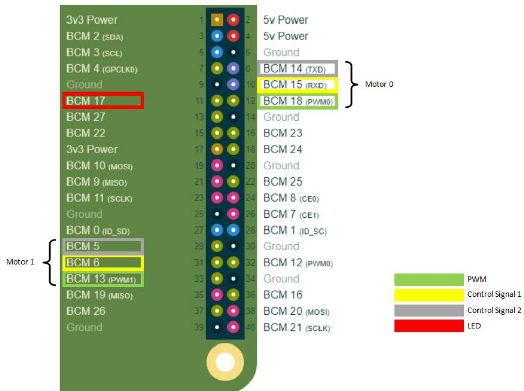
Figure 3.4.1: Pin placements as dictated by code. Labelled version of [3].
